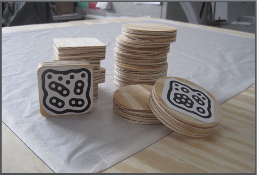
Figure 7. These symbols mark the objects that are tracked by reactIVision. Each symbol is unique.
